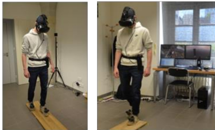
Figure 3. The participant on the plank is equipped with a tDCS cap, a VR helmet and two trackers attached to his feet. The computers in the room provided a 1st and 3rd person view of the participant's virtual environment in real time.
