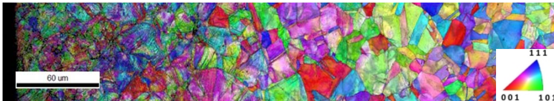
Fig. 1. Microstructure observation on the cross-section of the SMATed specimen.
