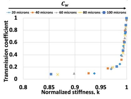
Fig. 22. Transmission coefficient versus the interface stiffness for different contact widths.
