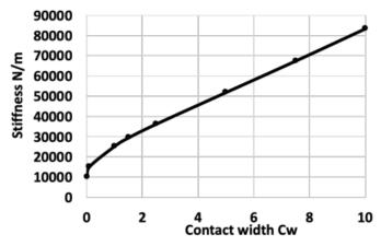
Fig. 15. Resulting contact stiffness versus the asperity/contact width
