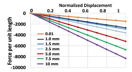
Fig. 14. Reaction force versus displacement for different asperity width configurations
