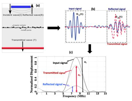
Fig. 5. (a) Solid-Solid interface (b) Time domain representation of input, reflected and transmitted waves (c) FFT or frequency domain representation of input, reflected and transmitted waves.
