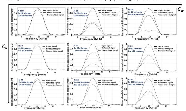
Fig. 16. Compilation of frequency domain plots showing difference in the transmission and reflection coefficients with their respective configuration changes.
