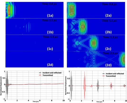
Fig. 6. Time lapse of wave travelling as it reaches the right end of the solid for (1) coarse mesh distribution (2) Fine mesh distribution Displacement magnitude (a) plotted for the coarse mesh distribution (b) plotted for the fine mesh
