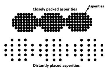
Fig. 2. Asperity distribution types in a contact when they are far apart and when they are closely placed
