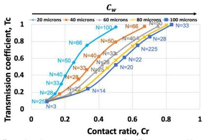
Fig. 18. Transmission coefficient plotted in comparison to contact ratio for different contact width configurations and number of asperities, Tc  $/ \infty$  Cr.
