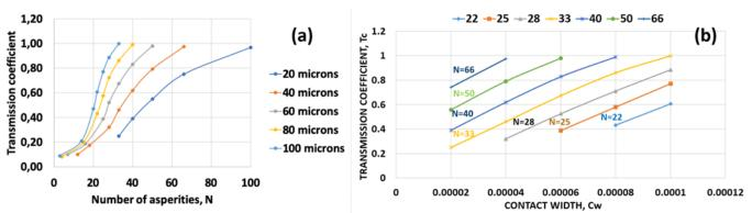
Fig. 17. a) Transmission coefficient plotted in comparison to change in contact width for different number of asperity
