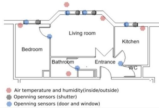
Figure 3: Industrial apartment plan and sensors location
