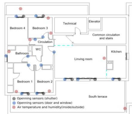
Figure 5: Contemporary flat plan and sensors location
