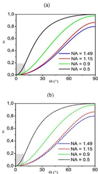
**Fig. 9.** Theoretical calculations of the DOP as a function of the dipole orientation  $\Theta$  for two configurations of collection: (a) with the beam stop limiting NA = 0.45, and (b) for a full collection. Four different objective numerical apertures are evaluated for each configuration. The grey zones correspond to dipoles which are oriented nearly vertical ( $\Theta = 0 - 10^\circ$ ).
