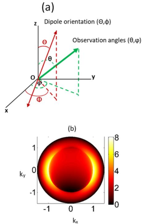
**Fig. 2.** (a) Schematic of the spherical coordinates defining the orientation of the dipole  $(\Theta, \Phi)$  and the direction of the observation  $(\theta, \varphi)$ ; (b) Simulated emission diagram on the Fourier plane of the objective of a dipole inclined  $15^\circ$  to the substrate.
