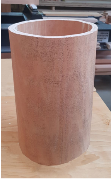
Fig. 2 Circular hollow tube made of green beech veneer
