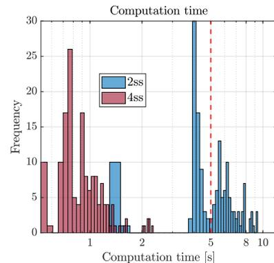
Fig. 6. The computation time of the NMPC in the two strategies. Note that red dash line depicts the sampling time which is  $T_s = 5$  seconds. The local MPC problems are synthesized and solved by using Casadi [10] and solver Ipopt, respectively.
