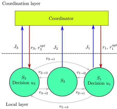
Fig. 1. Example of the hierarchical control architecture and the interconnection network between the subsystems. The presented sets correspond to this example are  $\mathcal{N} := \{1, 2, 3\}$ ;  $\mathcal{N}^{ctr} := \{1, 3\}$ ,  $\mathcal{N}_1 = \{2, 3\}$ ,  $\mathcal{N}_2 = \{1, 3\}$ ,  $\mathcal{N}_3 = \{1, 2\}$ .
