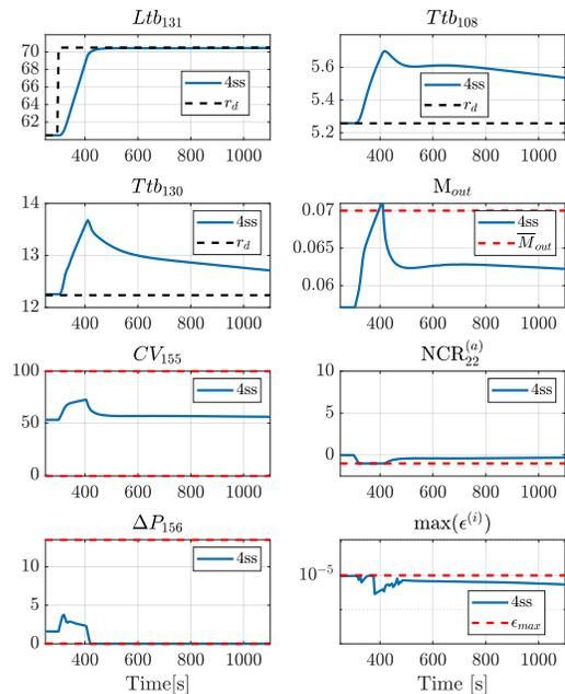
Fig. 5. The system behavior under the hierarchical control framework. In this scenario, the set-point of liquid helium level  $Ltb_{131}$  is changed at instant  $t = 300$ . This figures also shows the actuator behaviors in subplot(4,2,5), subplot(4,2,6) and subplot(4,2,7). Subplot(4,2,8) shows the maximum convergence error of fixed-point iterations  $\max(\epsilon^{(i)})$  founded in the grid  $\mathcal{G}$  of candidate setpoints at each time step.
