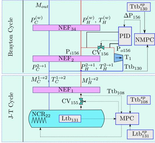
Fig. 2. Block diagram of the cold box plant.
