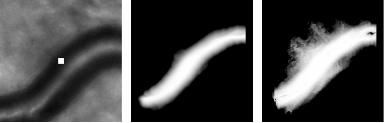
Figure 13: Left: Crop of the input image of Figure 7, with a pixel i marked as the center of the white square. Center: Neighborhood \mathcal{N}_i^k in the non binary-weighted co-circularity graph with k = 15 and parameters \sigma = 5 , p = 7 and \beta = \frac{\pi}{6} . Right: Neighborhood of the same pixel in the non binary-weighted graph with same parameters except \sigma = 2 . As we can see the two neighborhoods are not ordered and the one for \sigma = 2 is less accurate with respect to the underlying vessel shape.
