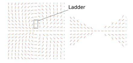
Figure 3: **Left:** a set of elements  $(u, \theta)$  co-circular to the central element  $(u_0, \theta_0)$  where  $u_0$  is the origin and  $\theta_0 = 0$  rad; **Right:** the elements from the left hand image that comply with the additional conic condition to avoid ladder configurations.
