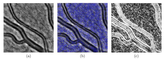
Figure 1: (a) A grayscale image, (b) its structure tensors  $T_{\sigma}$  for  $\sigma = 3$  pixels and (c) the corresponding anisotropy image. In (b) an ellipse is plotted every 15 pixels in both directions.
