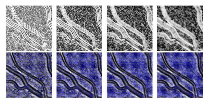
Figure 2: Anisotropy images (top row) associated with smoothed structure tensors  $T_{\sigma}$  (bottom row, subsampled every 15 pixels) for several values of  $\sigma$ . From left to right,  $\sigma = 1, 3, 5, 7$  pixels. The grayscale input image is the one shown in Figure 1 (a).
