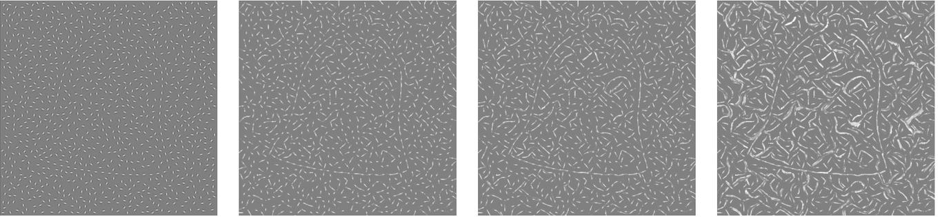
Figure 12: Input image and three closings  $\varphi_{W^k} = \varepsilon_W^k \delta_W^k$  for  $k = 1, 2, 3$  and  $W$  the adjacency matrix of the binary-weighted co-circularity graph obtained with parameters  $\sigma = 4$ ,  $p = 7$ ,  $\beta = \frac{\pi}{6}$  and  $\alpha = \frac{\pi}{20}$ .
