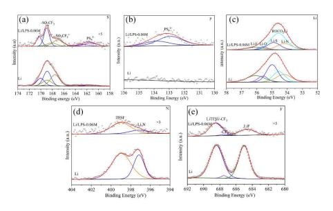
Figure 4. (a) S 2p, (b) P 2p, (c) Li 1s, (d) N 1s and (e) F 1s XPS spectra and the fitting results of the
