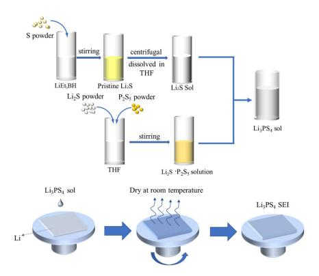
Schematic 1. Synthesis route of the Li<sub>3</sub>PS<sub>4</sub> sol and the preparation of the Li<sub>3</sub>PS<sub>4</sub> artificial SEI layer
