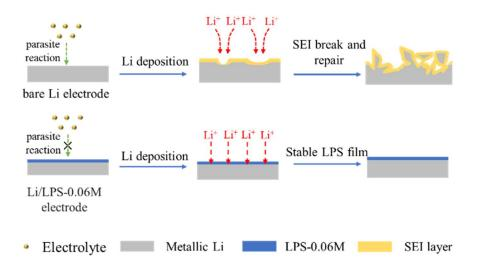
Schematic 2. Schematic of the bare Li and the Li/LPS-0.06M electrodes during the Li stripping and plating process.
