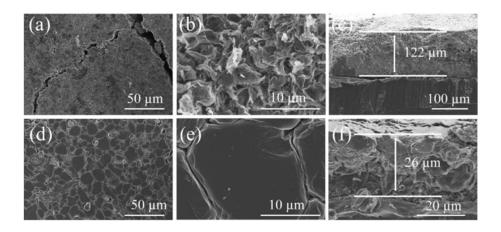
Figure 3. Morphology of the symmetrical cells with the bare Li and Li/LPS-0.06M electrodes after 500 h cycling at 1 mA cm<sup>-2</sup> and 1 mAh cm<sup>-2</sup>. (a, b) Top-view and (c) cross-sectional SEM images of the bare Li electrode. (d, e) Top-view and (f) cross-sectional SEM images of the Li/LPS-0.06M electrode.
