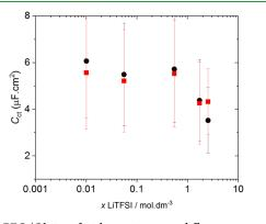
**Figure 8.** PEO/Oh interfacial capacitance at different concentrations of LiTFSI in the PEO. Circles and squares from data at 100 and 80  $^{\circ}$ C, respectively.
