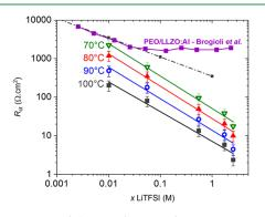
**Figure 7.** Variation of the PEO/Oh interface resistance at different salt concentrations for different temperatures from 70 to 100 °C. Literature values from Brogioli et al. at 70 °C are also included.<sup>57</sup> The dotted/dashed line represents a power law of -0.5.
