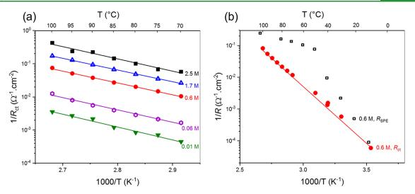
**Figure 6.** Arrhenius plots displaying 1/R versus 1000/T for (a) the interfacial charge transfer at the PEO/Oh interface at different LiTFSI concentrations for a temperature range of 100-70 °C and (b) comparison of the bulk PEO/LiTFSI-0.6M resistance (thickness of  $102 \ \mu\text{m}$ ) with charge transfer resistance at the PEO/LiTFSI-0.6M/Oh interface for a temperature range of 100-10 °C.
