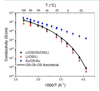
Figure 3. Arrhenius plot of the conductivities (high-frequency contribution) of electrolytes OS (red triangles) and Oh (blue diamonds) and the sandwich OS/Oh/OS (black squares) along with the theoretical values of OS/Oh/OS (black line) using eq 1.
