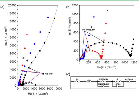
Figure 1. (a) Nyquist plots of the SS/OS/SS (red triangles), Au/Oh/Au (blue diamonds), and SS/OS/Oh/OS/SS (black squares) cells measured at 20 °C. In addition, the subtraction (black open diamonds) of the SS/OS capacitive contribution from the spectrum of SS/OS/Oh/OS/SS is also displayed. Markers: experimental values; solid line: fitted values, using the equivalence circuit displayed in (c). (b) Zoom on the HF region of the plot (a).
