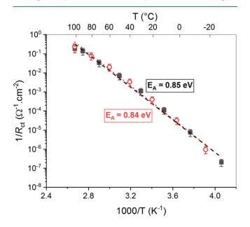
**Figure 5.** Arrhenius plots of the **Oh/OS** interfacial resistance obtained through a blocking electrode configuration (filled squares) from the cell SS/**OS**/**Oh**/**OS**/SS and a nonblocking electrode configuration (open circles) from the cell Li/**OS**/**Oh**/**OS**/Li.
