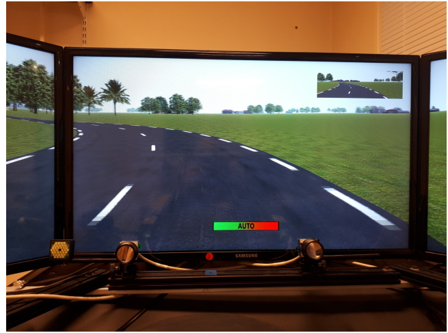
Fig. 4. Centre screen of the simulator displaying the progressive bar while in autonomous mode
