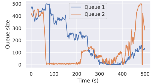
Fig. 6: Example of the evolution of the two bottleneck queue lengths at s1 and s2 for two different time periods.
