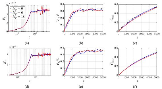
**Figure 5.** The effect of rigid stones on the flow field as a function of the number,  $N_p$ , for  $R_s = 2$  and Pe = 500. Kinetic energy, entrapped fluid volume when Q > 0, and the clearance rate of a passive tracer are shown in columns one to three, respectively. The top and bottom panels correspond to Re = 250 and Re = 500, respectively.
