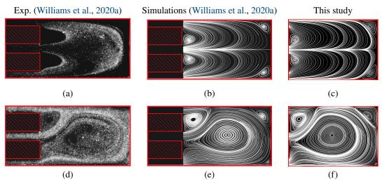
**Figure 8.** Direct comparison of the streamlines from our numerical predictions, third column, with both experimental and simulation results reported by Williams et al. (2020a), first and second columns, for a two-dimensional cavity characterised by b = 1.933, h = 4.2835, and cavity-length  $\alpha = 21.7$  (here,  $\alpha$  stands for the nondimensional length of the rectangular cavity). Panels (a)-(c) and (d)-(f) represent the flow dynamics with Re = 7 and Re = 34, respectively.
