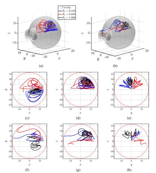
**Figure 3.** Trajectories of single rigid stones up to t = 5000. Panels (a) and (b) correspond to a threedimensional representation of the trajectories for Re = 250 and Re = 500, respectively. Panels (c)-(h) correspond to the projection of the trajectory onto the xy-, xz- and yz-plane for Re = 250 (middle panels) and Re = 500 (bottom panels), respectively. The red circles correspond to the limits of the cavity, where the center of the spherical cavity corresponds to  $\mathbf{x} = (0, 0, 0)$ .
