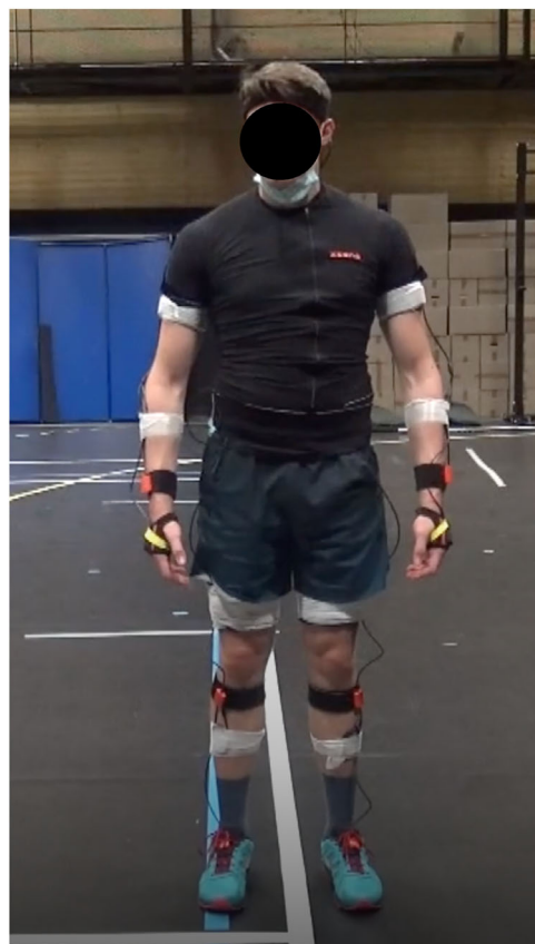
FIGURE 1 Subject equipped with inertial measurement units (IMUs). Sensor's locations: Hands, lower arms, upper arms, feet, lower legs, upper legs, pelvis and sternum
