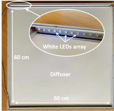
Fig. 8. Typical LED light fixture used for indoor illumination (Sylvania START Panel Flat UGR19 600x600 Neutral White). This typical panel consists of 144 total mid-power LEDs and outputs a luminous flux of 3500 lm.
