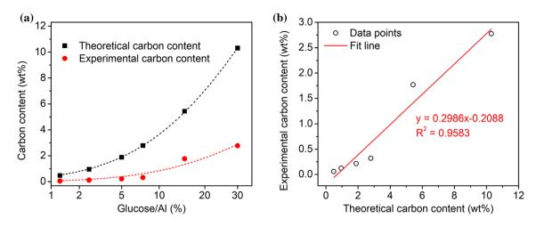
Figure 3 a Experimental and theoretical contents *vs* the initial glucose/Al mass ratio. b Experimental carbon content *vs* theoretical carbon content. The fit lines are guides to the eye.
