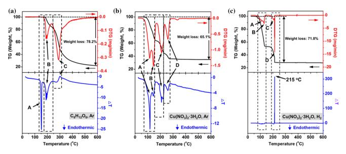
Figure 4 TG (black), DTG (red) and DTA (blue) curves for a  $C_6H_{12}O_6$  in Ar gas atmosphere, b  $Cu(NO_3)_2 \cdot 3H_2O$  in Ar gas atmosphere and c  $Cu(NO_3)_2 \cdot 3H_2O$  in  $H_2$  gas atmosphere.
