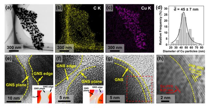
**Figure 8 a** BF STEM image of a GNS Cu hybrid layer and b, c the corresponding EDS mapping; d the Cu particles diameter distribution. e, f HRTEM images showing the GNS layer bridging
