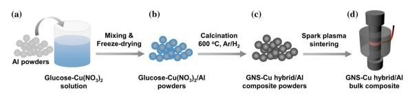
Figure 1 Schematic illustrations for the fabrication process of GNS Cu/Al composites.
