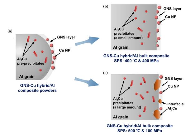
Figure 13 Schematic diagram of composition and microstructure for **a** the GNS Cu/Al composite powder, **b** the sample sintered in the S 4 4 conditions and **c** the sample sintered in the S 5 1 conditions.
