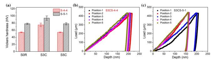
Figure 14 a Vickers microhardness (HV) for the S0R, S3C and S5C samples sintered in the S 4 4 and S 5 1 conditions; nanoindentation load depth curves for b S3CS 4 4 and c S3CS 5 1.
