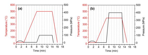
Figure 2 Spark plasma sintering cycles: a 500 °C and 100 MPa (conditions S 5 1) and b 400 °C and 400 MPa (conditions S 4 4).
