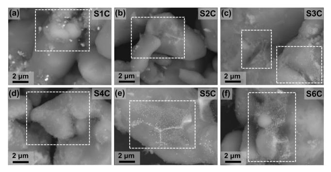
Figure 7 SEM images (BSE mode) of the S1C S6C GNS Cu/Al composite powders. The boxed areas indicate some GNS Cu hybrid layers.
