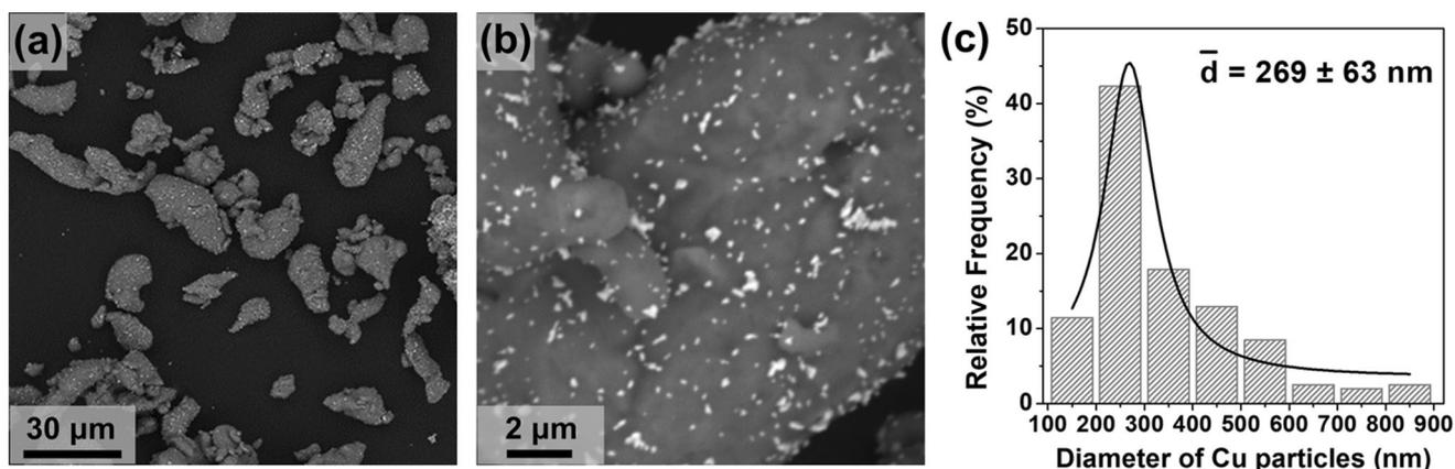
**Figure 9** a, b SEM images (BSE mode) of the S0R Cu/Al composite powder; c diameter distribution of the Cu particles located at the surface of the Al grains.
