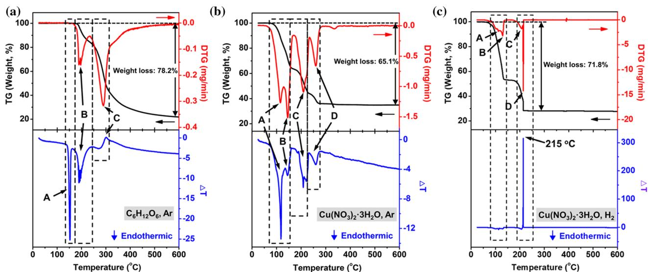
**Figure 4** TG (black), DTG (red) and DTA (blue) curves for a  $C_6H_{12}O_6$  in Ar gas atmosphere, b  $Cu(NO_3)_2 \cdot 3H_2O$  in Ar gas atmosphere and c  $Cu(NO_3)_2 \cdot 3H_2O$  in  $H_2$  gas atmosphere.
