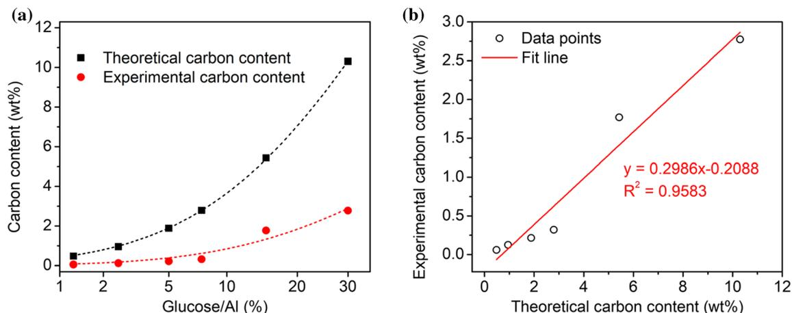
**Figure 3** a Experimental and theoretical contents vs the initial glucose/Al mass ratio. b Experimental carbon content vs theoretical carbon content. The fit lines are guides to the eye.
