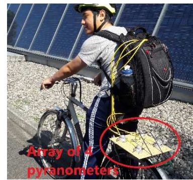
Figure 10 Experiment to measure the potential irradiation as received by our system during a bike ride
