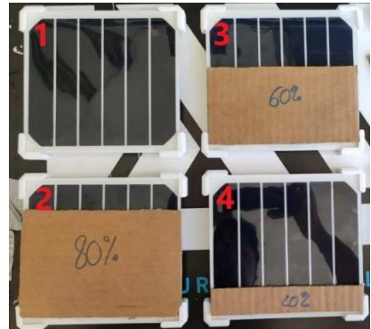
Figure 6 Test setup to simulate the effects of partial shading
