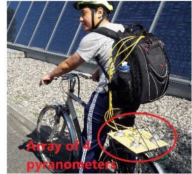
Figure 10 Experiment to measure the potential irradiation as received by our system during a bike ride
