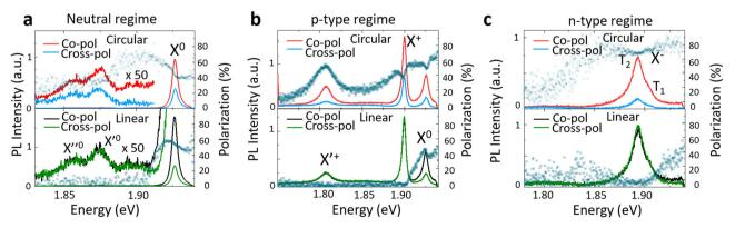
**Fig. 3 Polarization behaviour of the photoluminescence.** Polarization-resolved photoluminescence (PL) emission under circularly polarized excitation and linearly polarized excitation for different gate voltages, +3V (**a**), +30 V (**b**) and -20 V (**c**). Here the PL components co-polarized and cross-polarized with respect to the laser are denoted by co-pol and cross-pol, respectively. Also shown is the energy-resolved degree of PL polarization (blue dots).
