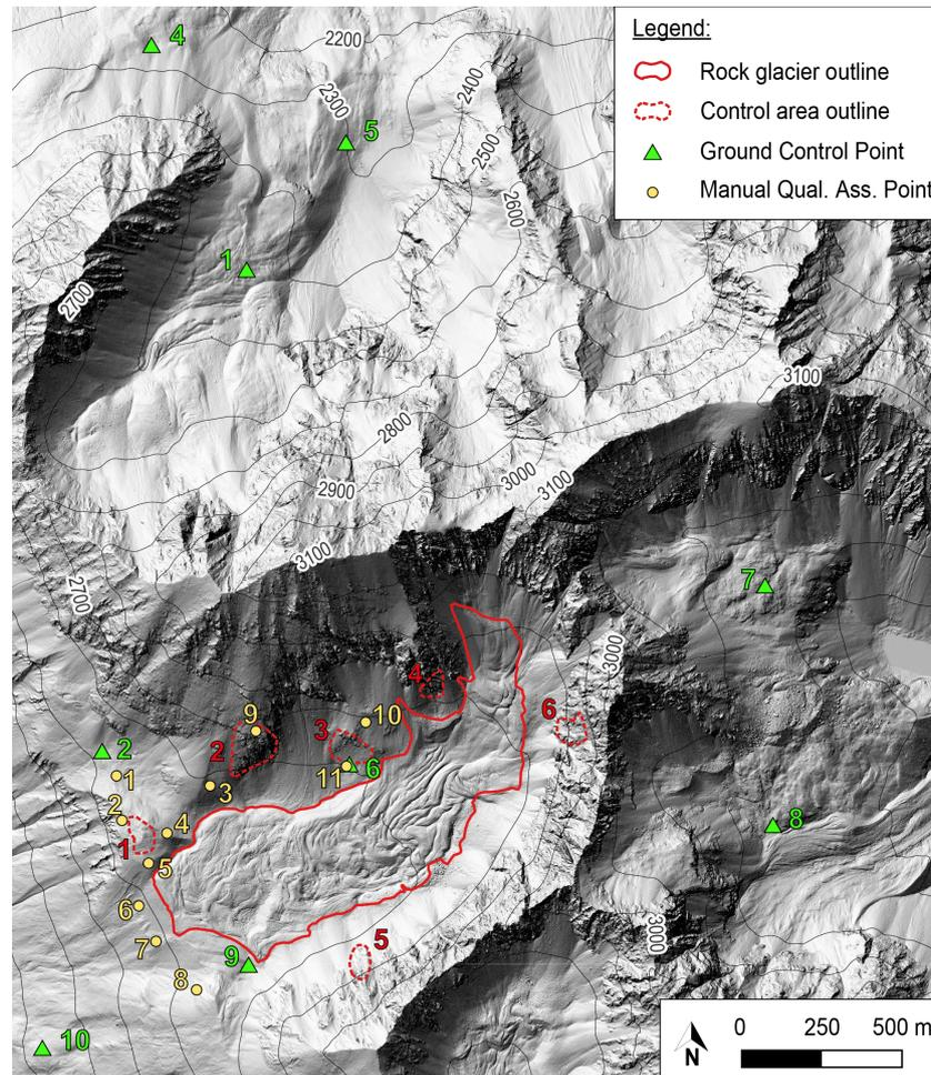
**Figure A1.** Map showing the location of the ground control points, the control areas, and the manual control points used in the remote sensing analysis. Hillshade DEM has been produced from high-resolution lidar DSM (0.5 m resolution) survey realized by SINTEGRA (17 August 2012).
