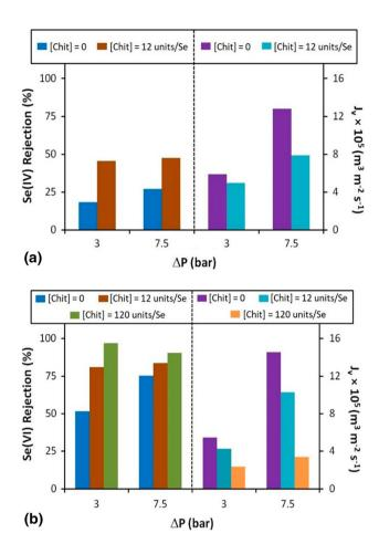
**Fig. 9** Rejection and permeation flux obtained by ultrafiltration of solutions containing 1.7 mmol/L of **a** Se(IV) and **b** Se(VI) with and without chitosan at pH 4. CERAM 60 membrane, molecular weight cut off: 8 kDa
