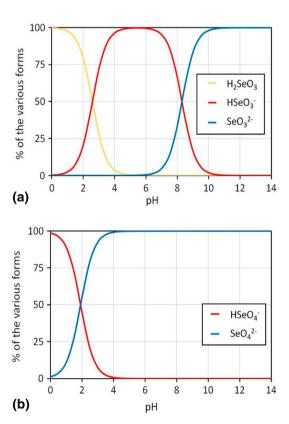
**Fig. 8** Speciation distribution of selenium forms versus pH. **a** Se(IV) and **b** Se(VI). At acidic pH, Se(IV) is either neutral selenious acid and/or monovalent anion (hydrogen selenite). At basic pH Se(IV) is either monovalent anion (hydrogen selenite) and/or in divalent anion (selenite ions). Se(VI) is mainly in the form of divalent anion (selenite ion) with a pH above 3.5
