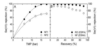
**Fig. 6** Rejection of Se(VI) with nanofiltration/reverse osmosis membranes versus **A** transmembrane pressure (TMP) and **B** recovery. Sources: A) is adapted from Malhotra et al. (2020): Se(VI) 1600  $\mu$ g/L and pH 8; B) is adapted from Chung et al. (2010): S(VI) 326  $\mu$ g/L, pH 7.2 and pressure 8 bar
