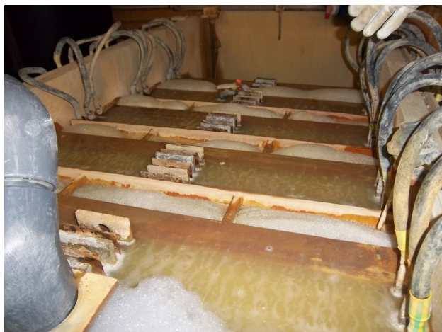
Fig. 3 An electrocoagulation unit at the industrial scale. Electrocoagulation is a well-known technique for the treatment of several metals and metalloids present in water and wastewater, in particular for selenium and arsenic, for example in the mining industry. Briefly, the process uses a metallic cation as a coagulant in an electrochemical reaction involving iron or aluminum electrodes as anodes; when a current is applied to electrodes in wastewater, the metal anode is oxidized and cations are released to the effluent, which then forms hydroxide precipitates
