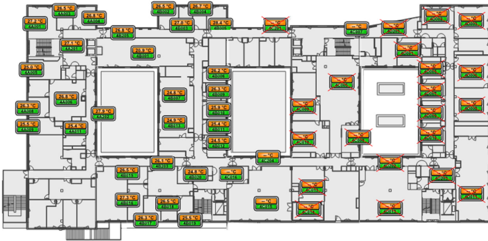
Figure 6: Temperature monitoring on each zone; example of the 4th floor.
