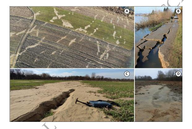
Figure 14: Examples of liquefaction following the Petrinja earthquake: (A) aerial view from drone at Letovanić (area 4 on Figure 15); (B) lateral spreading along Kupa river embankment at Letovanić (area 4 on Figure 15); (C) crack with sand ejecta in the alluvial plain of the Sava river; (d) sand and gravel ejecta of different provenance with presence of shells close to Kupa river.
