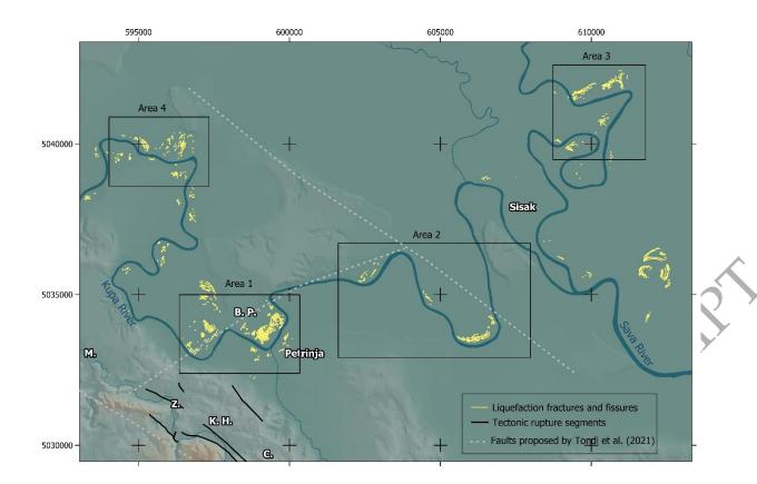
Figure 15. Map of liquefaction-related fissures in the epicentral area (field-checked and remote sensing), around Petrinja and Sisak. Fissures were drawn based on a visual analysis of drone and satellite images (some available on Google Earth). Areas 1 to 4 refers to focused maps and pictures provided in Suppl. Mat. S3. B. P.: Brest Pokupski. Fault lines as inferred by Tondi et al. (2021) are shown in white dashed lines for comparison.
