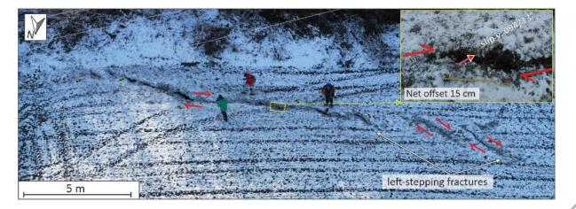
Figure 10. Aerial view (drone survey) of a ~20 m-long surface rupture on alluvial fan gravels mapped southwest of Križ Hrastovački on the Križ section (section 3 on Fig. 7, "Site 8" in database). Surface faulting occurred as a continuous rupture, striking 120°, or as a set of left-stepping en échelon ruptures. The maximum coseismic offset, measured between well-preserved piercing points, is ~15 cm.
