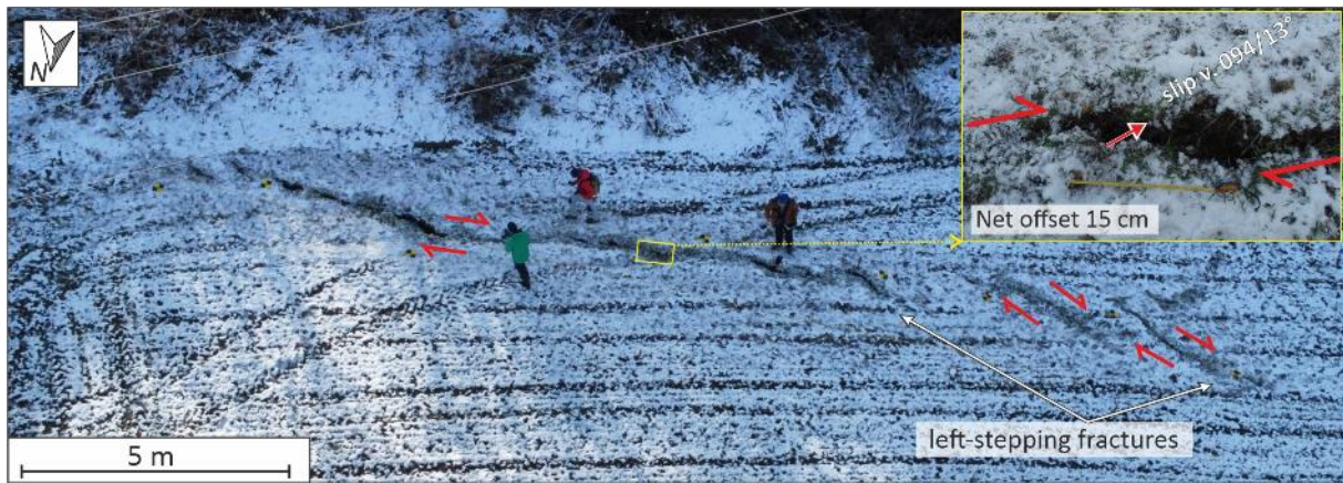
Figure 10. Aerial view (drone survey) of a ~20 m-long surface rupture on alluvial fan gravels mapped southwest of Križ Hrastovački on the Križ section (section 3 on Fig. 7, “Site 8” in database). Surface faulting occurred as a continuous rupture, striking 120^\circ , or as a set of left-stepping en échelon ruptures. The maximum coseismic offset, measured between well-preserved piercing points, is ~15 cm.
