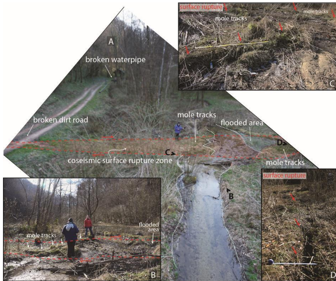
Figure 9: Surface faulting south of Križ Hrastovački on the Župić section (section 2 on Fig. 7; “site 5” in database). A continuous, approximately 55 m long, coseismic surface rupture zone was observed crossing Kladnjik stream, a tributary of the Utinja River, and the nearby field and dirt road. Coseismic disjunction between a concrete reservoir and a PVC water pipeline transversal to the faulting was reported by locals a few tens of meters west of the surface ruptures (see arrow in main picture A). Ruptures have a left-stepping arrangement with mole tracks (pictures B and C) and a gentle warp of the ground across an approximately 5 m wide zone parallel to the fault. A wide zone of flooding occurs on the left bank of the stream as a consequence of dextral offset (main picture A). The creek shows a cumulative dextral offset up to 2 m. The 2020 coseismic offset can be reconstructed by using singularities in its edges as piercing points: a minimum coseismic lateral motion of 0.3-0.4 m has been estimated. These values are affected by uncertainty in the reconstruction of the original edges that are eroded and presently modified by the mole tracks and because they were surveyed about 2 months after the earthquake.
