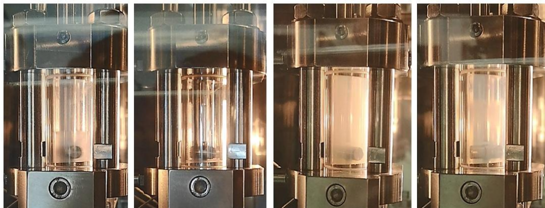
Figure 3. Transition of a fluid from subcritical to the critical state on density increase. From left to right: classical vapor liquid mixture (the two phases are perfectly separated by a thin meniscus); saturated vapor phase (the vapor-liquid interface disappear at the bottom of the optical cell); saturated liquid phase (the vapor-liquid interface disappear at the top of the optical cell. The meniscus becomes thicker and thicker and the liquid phase become cloudy and milky); critical opalescence (vapor-liquid interface disappear at the center level of optical cell, and the meniscus become darkness and occupies the entire optical cell).
