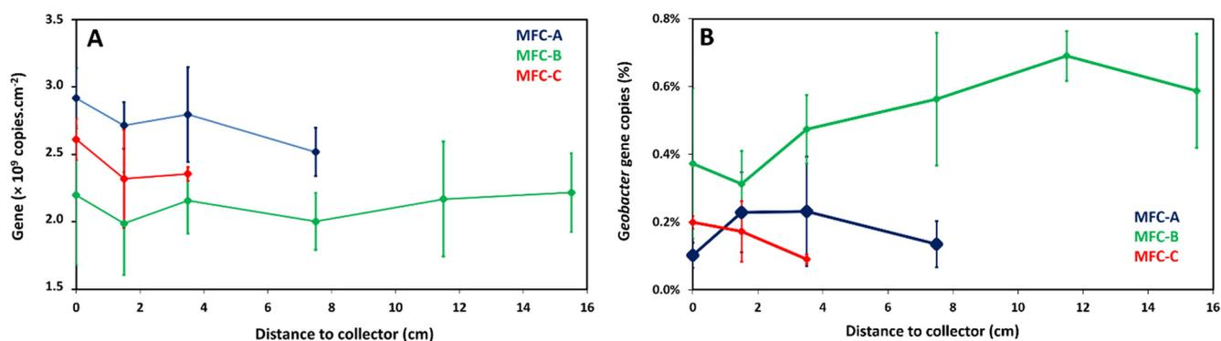
**Figure 3.** Distribution as a function of the distance from the collector of all bacteria (quantified by qPCR as gene copies number per anode cm<sup>2</sup>) (A) and of relative abundance of *Geobacter* (determined by qPCR ratios of *Geobacter* to total bacteria) (B).
