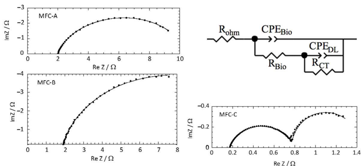
**Figure 5.** Nyquist plots for MFC-A, MFC-B, and MFC-C. Experimental (dots) and fitted data (lines) are presented. Electrical equivalent circuit used to fit anode impedance spectra.  $R_{ohm}$ : electrolyte resistance;  $R_{CT}$ : charge transfer resistance;  $R_{Bio}$ : biofilm resistance;  $CPE_{DL}$  and  $CPE_{Bio}$ : constant phase elements respectively from double layer and biofilm.
