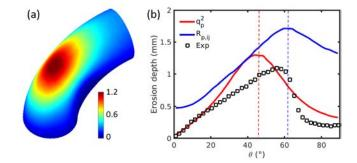
**Figure 2:** (a) Contour of erosion depth with the particle turbulence model  $q_p^2$ ; (b) Erosion depth profiles on the elbow extrados for two different particle turbulence models, the dashed lines correspond to the erosion peak location.
