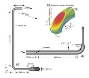
**Figure 1:** (a) and (b) Experiment set-up of Solnordal et al. (2015); (c) Contour of erosion depth after passage of  $200 \ kg$  sand.
