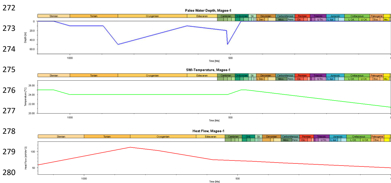
281 Fig. 3. The thermal boundary condition assessment for Magee-1 well including: (top) 282 the paleowater depth (PWD, in meter) and (middle) the sediment-water interface 283 temperature (SWIT, in °C), and (bottom) the paleo-heat flow (HF, in mW/m 2 ). The basal 284 heat flow values were specified for each geologic event using the present-day analogs 285 and extrapolated through time (Allen and Allen, 1990).
