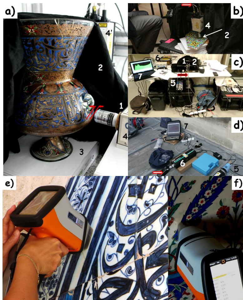
Fig. 12: On-site analysis with a mobile Raman set-up. Measurements are made in Museum storage rooms: a) horizontal analysis, b) analysis from the top with a mobile support, c) view of the whole set-up, or d) on the roof of Sainte-Chapelle Palatine Church, Paris; 44 1, long working distance microscope objective (the distance between the object surface and the front lens is indicated); 2, black textile; 3, paper rams to adjust the height of the object and to suppress vibrations; 4, remote optical head; 5, Raman spectrometer and CCD detector (in blue); 6, laser; 7, computer; e) and f) examples on measurements with an handheld XRF pistol: in e) the screen allows controlling the analysed spot; the instrument gives after collecting data (a few minutes) a first look of the elemental composition.
