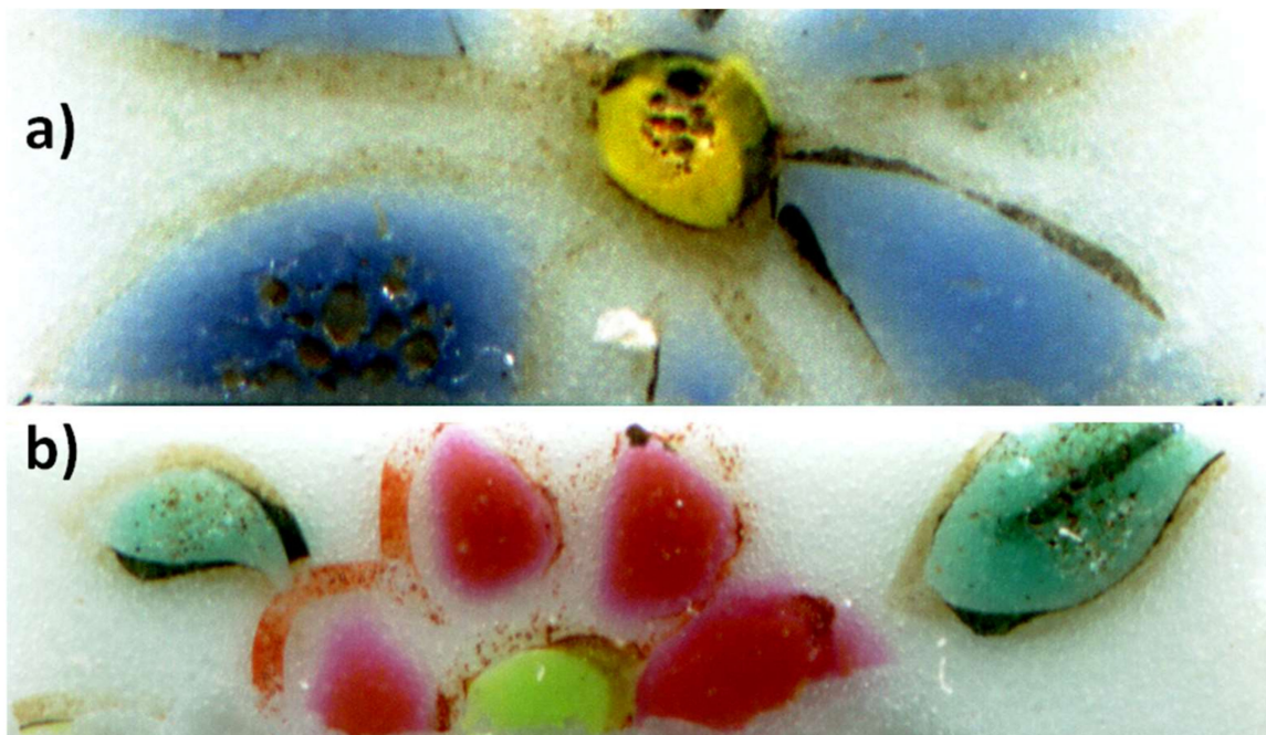
Figure 3. Detail view of the décor of Rose plate ( 20 \times 4 \text{ mm}^2 , each, see Appendix A, Figure A1e): yellow, blue, red, pink, green, black overglazes and colorless glaze of areas depicting blue (a) and red (b) flower (see corresponding elemental composition in Tables 2 and 3).
