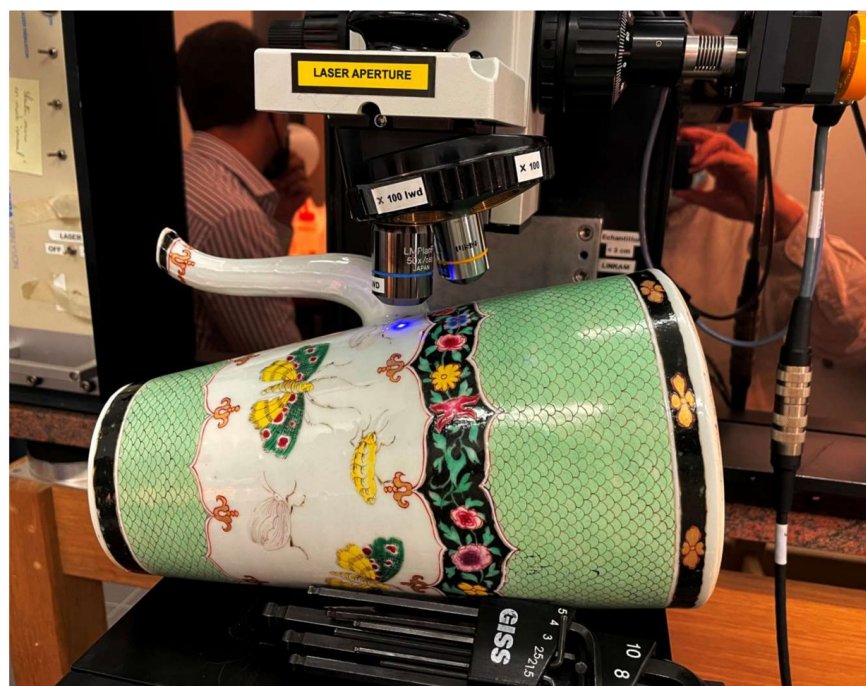
Figure 1. Coffee pot with Prunk's design undergoing Raman analysis using a long working distance microscope (50×) objective. The analyzed spot is much smaller than the white halo.
