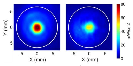
Figure 7. Ultrasound temporal-average intensity distribution  $I_{\text{TA}}$  [mW/cm<sup>2</sup>] without (left – Fig. 3a) and with (right – Fig. 3b) the Petri dish for 2.25 MHz-transducer at  $z_f = 39$  mm. The white circle represents the area of the transducer.
