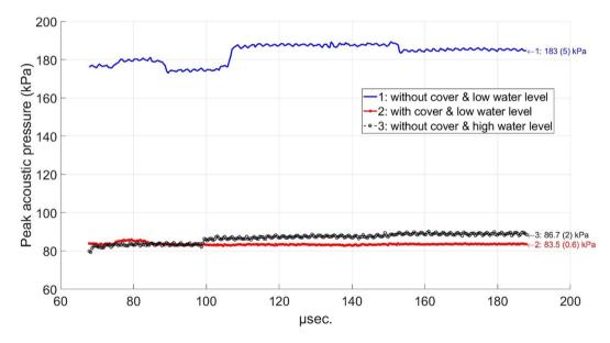
Figure 9. Moduli of the Hilbert transform of the transmitted RF-signals between the 2.25 MHz-transducer and the hydrophone in horizontal position and a low water level above the Petri dish, and the hydrophone in vertical position and a high water level. On the right, the mean values and standard deviations are mentioned.
