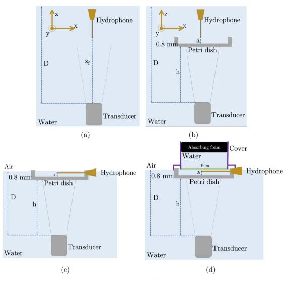
Figure 3. Schematic drawings of *high water level configuration* (a) without and (b) with the Petri dish and *low water level configuration* (c) without and (d) with the anti-reflection cover.
