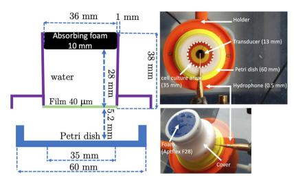
Figure 1. Schematic drawing and pictures of the Petri dish/anti-reflection cover set.
