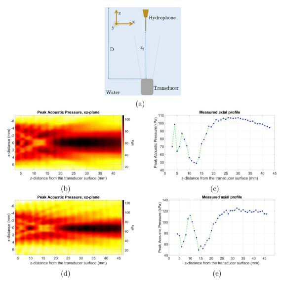
**Figure 4.** Calibration configuration (a). Pressure distribution in *xz*-plane for the 1 MHz-transducer for free field (b) and along the beam axis (c). Pressure distribution in *xz*-plane for the 2.25 MHz-transducer for free field (d) and along the beam axis (e).
