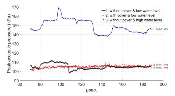
Figure 8. Moduli of the Hilbert transform of the transmitted RF-signals between the 1 MHz-transducer and the hydrophone in horizontal position and a low water level above the Petri dish, and the hydrophone in vertical position and a high water level. On the right, the mean values and standard deviations are mentioned.
