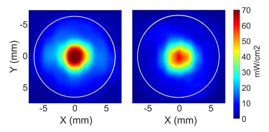
Figure 6. Temporal-average intensity  $I_{\text{TA}}$  [mW/cm<sup>2</sup>] distribution without (left – Fig. 3a) and with (right – Fig. 3b) the Petri dish for 1 MHz-transducer at  $z_f = 28$  mm. The white circle represents the area of the transducer.
