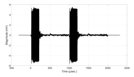
Figure 5. Example of RF-signal recorded by the hydrophone at  $z_f = 28$  mm. Configuration: 1 *MHz-transducer*, high water level, vertical position of the hydrophone.
