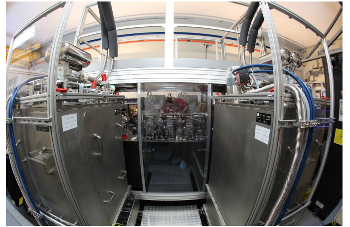
Fig. 2. Fish-eye view of the backside of MATISSE in the VLTI laboratory. The two stainless-steel grey structures are the two cryostats, the left one housing the N band cold optical bench (COB) and detector, and the right one housing the L and M band COB and detector.
