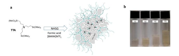
**Figure 1**. (a) Schematic synthesis of ionosilica ionogels; (b) photograph of the ionosilica ionogel monoliths with different IL volumes.
