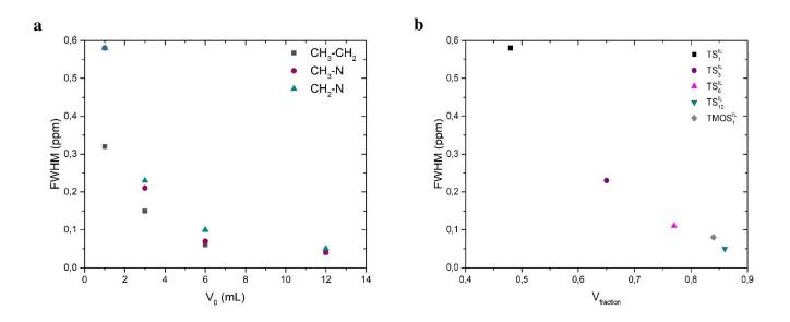
Figure 5. (a) variation of the FWHM as a function of the quantity of confined IL for three characteristics <sup>1</sup>H signals of the IL; (b) variation of the FWHM of the CH<sub>2</sub>-N signal as function of the IL  $V_{\text{fraction}}$  in the **TS**<sup>IL</sup><sub>x</sub> and **TMOS**<sup>IL</sup><sub>1</sub> monoliths.
