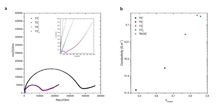
Figure 7. (a) Nyquist plots obtained for the different  $TS_x^{IL}$  samples using broadband dielectric spectroscopy (BDS), (b) the variation of the conductivity of the  $TS_x^{IL}$  and  $TMOS_1^{IL}$  materials as function of the IL V<sub>fraction</sub>.
