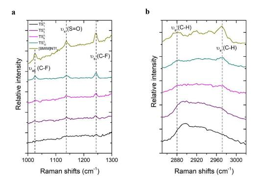
Figure 6. Raman spectra of the  $TS_x^{IL}$  ground monoliths and the pure IL in the range of (a) 1000-1300 cm<sup>-1</sup> and (b) 2850-3100 cm<sup>-1</sup>.
