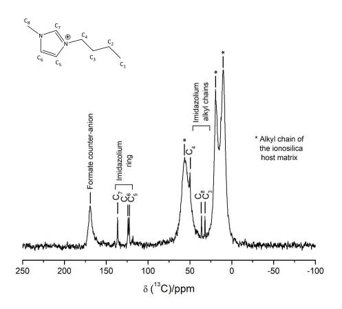
**Figure 2**. Solid-state <sup>13</sup>C CP NMR spectrum of the I<sup>2</sup>SG monolith synthesized in the presence of 6 mL of IL(**TS**<sub>6</sub><sup>IL</sup>). NMR shifts (ppm): TS alkyl chain (9.9, 19.2 and 56.7 ppm); C<sub>3</sub>(32.1 ppm); C<sub>4</sub> (50.1 ppm); C<sub>5</sub> (122.6 ppm); C<sub>6</sub> (123.9 ppm); C<sub>7</sub> (136.4 ppm); C<sub>8</sub> (36.0 ppm) and formate counteranion (166.7 ppm).
