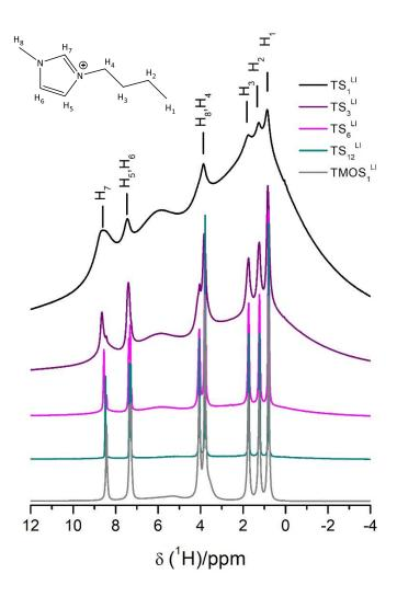
Figure 4. <sup>1</sup>H solid-state MAS NMR spectra of ground  $TS_x^{IL}$  and  $TMOS_1^{IL}$  monoliths respectively ( $v_{MAS} = 24 \text{ kHz}$ ).
