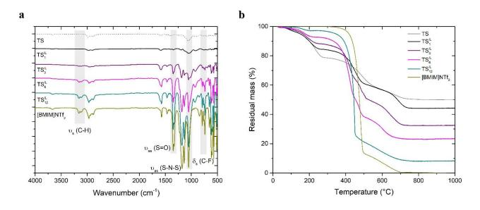
**Figure 3.** (a) FT-IR spectra and (b) TGA curves of  $I^2SG$  monoliths  $\mathbf{TS}_{\mathbf{x}}^{\mathbf{IL}}$  (where x is the initial volume of IL), neat TS monolith and IL.
