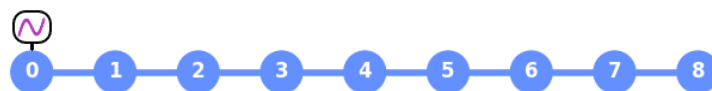
Figure 1: A linear chain of nine qubits with open boundary conditions. The uniform color of the qubits indicate that their lab frequencies are all identical [ \Delta = 0 in Eq. (19)]. Qubit 0 on the left edge is being driven periodically as in Eq. (20), and the qubits interact with their nearest neighbors by a “flip-flop” (XY) interaction term as in Eq. (21).
