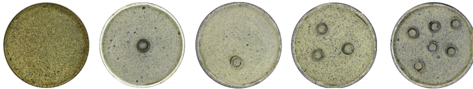
Figure 1: Experimental samples: S_0 , S_{1c} , S_1 , S_3 and S_6 . Underscript c indicates that the inclusion is centered.
