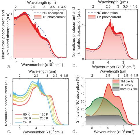
**Figure 4.** Broadband absorption in the short and mid-wave infrared. a,b) Simulated NC absorption and experimental photocurrent spectra under TE (resp. TM) polarization, at 80 K. c) Experimental unpolarized photocurrent spectra at various temperatures. d) Simulated absorption spectra for the bare NC film and the same film introduced in our multi-resonant geometry.
