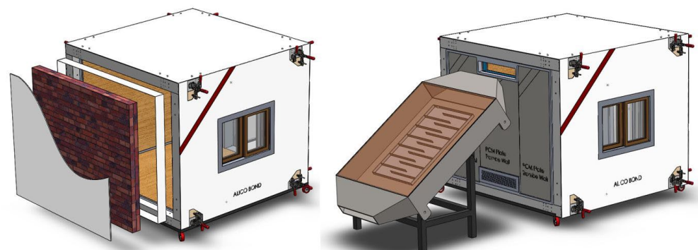
Figure 25. Brick wall sections for application P1 (to the left) and Solar air heater installed with necessary edits of the side wall of ThermoGreen® (to the right).
