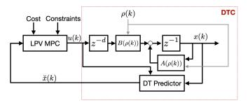
Fig. 1. Proposed LPV MPC with explicit dead-time compensation.
