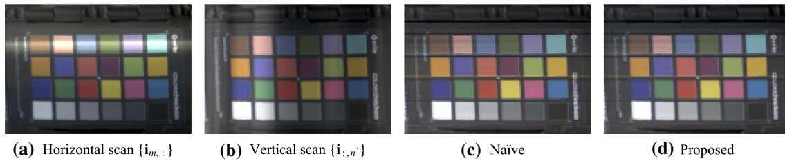
Fig. 4 The RGB images synthesized from the scanned images and the mitigated results. The illumination variations appear in the scanned images. One column of the vertical scan was used for mitigating the variation in the horizontal scan image
