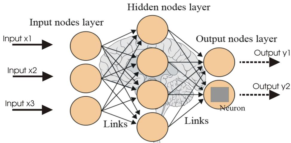
Figure 5: Artificial Neural Network Structure.
