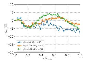
Fig. 9: Influence of the Reynolds number  $Re_{\lambda}$  on the relative energy error  $e_{rel}$  after one iteration of Parareal with spatial coarsening  $(N=4,\,N_{\Delta_t,\hat{\mathcal{G}}}=20,\,\text{injection}$  and  $7^{th}$ -order interpolation as transfer operators).
