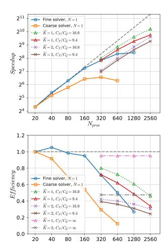
Fig. 5: Simulated speedup (top) and parallel efficiency (bottom) of Hybrid (fine and coarse solvers), and of Parareal with spatial coarsening after  $(\hat{K}=1,2)$  iterations.
