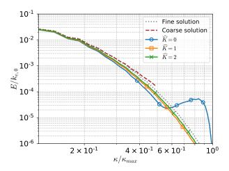
Fig. 6: Energy spectra after  $\hat{K}$  iterations of Parareal with spatial coarsening at  $t_{end}$   $(N=4, N_{\Delta_t, \hat{\mathcal{G}}}=20, \text{trilinear})$  interpolation and injection as transfer operators).
