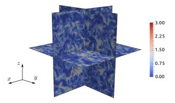
Fig. 2: Plane cuts of local turbulent kinetic energy  $k_{e,loc}/k_{e,0}$  for  $Re_{\lambda,0}=322$   $(k_{e,loc}=\frac{u.u}{2})$ .
