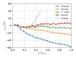
Fig. 8: Influence of the interpolation operator on the relative energy error after one iteration of Parareal with spatial coarsening ( $N=4,~N_{\Delta_t,\hat{\mathcal{G}}}=20$ , injection as restriction operator).
