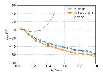
Fig. 7: Influence of the restriction operator on the relative energy error after one iteration of Parareal with spatial coarsening ( $N=4,\ N_{\Delta_{I},\hat{G}}=20$ , trilinear interpolation).
