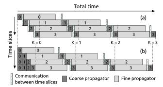
Fig. 1: Execution diagram of Parareal with pipelining (top) and with improved pipelining (bottom). Three iterations of Parareal (K=3) on four time slices (N=4) are considered. The end of each Parareal iteration is indicated by a dotted line. Time-slices are numbered from 0 to 3, each line corresponds to one process of Parareal.
