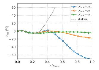
Fig. 10: Influence of  $N_{\Delta_t,\,\hat{\mathcal{G}}}$  on the relative error on the energy spectrum after one iteration of Parareal with spatial coarsening (N=4, injection and  $7^{th}$ -order interpolation as transfer operators).
