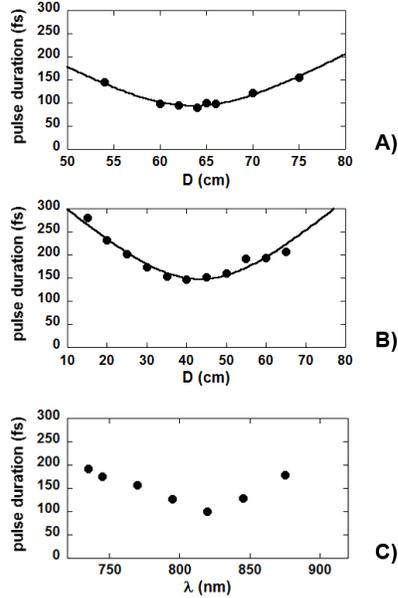
Fig. 3. Temporal compensation. Pulse duration (fs) as a function of the AOM-AOD distance ( $D$ ) measured: A) at 820 nm for the large scanner 1; B) at 840 nm for the small scanner 2. The lines are fit to the data using Eq.3. C) Pulse duration (fs) measured as a function of the wavelength  $\lambda$  (nm) for the scanner 1 ( $D=63$ cm).
