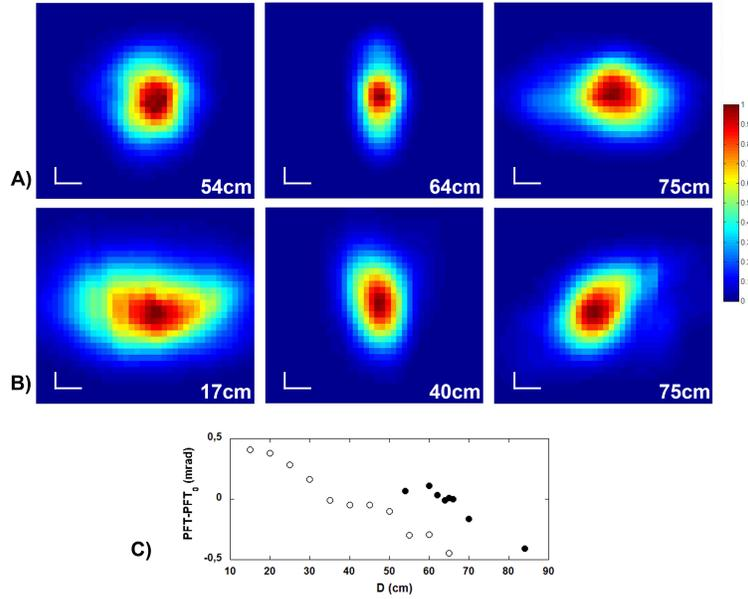
Fig. 4. Spatio-temporal distortions. GRENOUILLE traces measured for 3 AOM-AOD distances: A) for the scanner 1 ( $D=54\text{cm}$ ,  $D=64\text{cm}$  and  $D=75\text{cm}$ ) B) for the scanner 2 ( $D=17\text{cm}$ ,  $D=40\text{cm}$  and  $D=75\text{cm}$ ). C) Pulse front tilt as a function of the distance  $D$  for the scanner 1 ( $\bullet$ ) and for the scanner 2 ( $\circ$ ). Horizontal bar: 100fs, vertical bar: 1nm.
