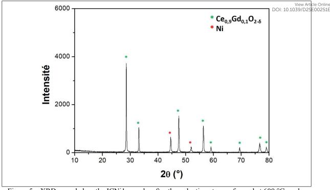
Figure 5 – XRD recorded on the ICNi1 sample, after the reduction step performed at 600 °C, under  $H_2/3\%H_2O$  gas flow, and the polishing of the current collector layer
