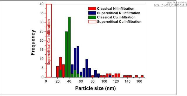
Figure 6. Histograms of the particles size distribution for each infiltration route
