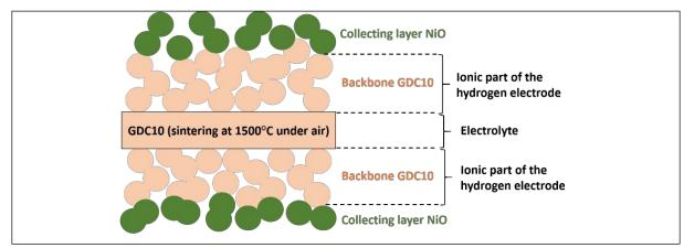
Figure 1. Scheme of a symmetrical hydrogen electrode before catalyst infiltration
