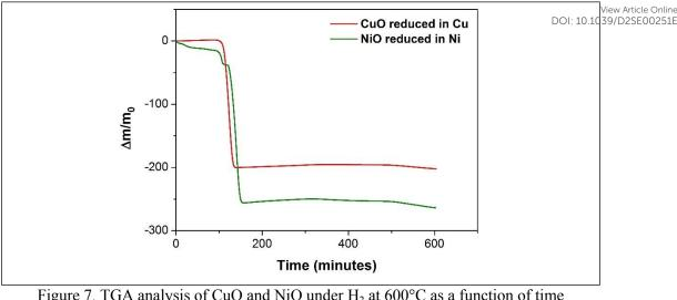
Figure 7. TGA analysis of CuO and NiO under H<sub>2</sub> at 600°C as a function of time
