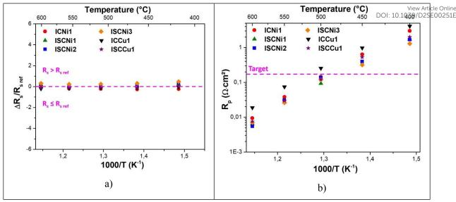
Figure 8. Arrhenius plots of series (a) and polarization (b) resistances measured on symmetrical cells (nickel or copper nitrate infiltration in a porous GDC10 backbone)
