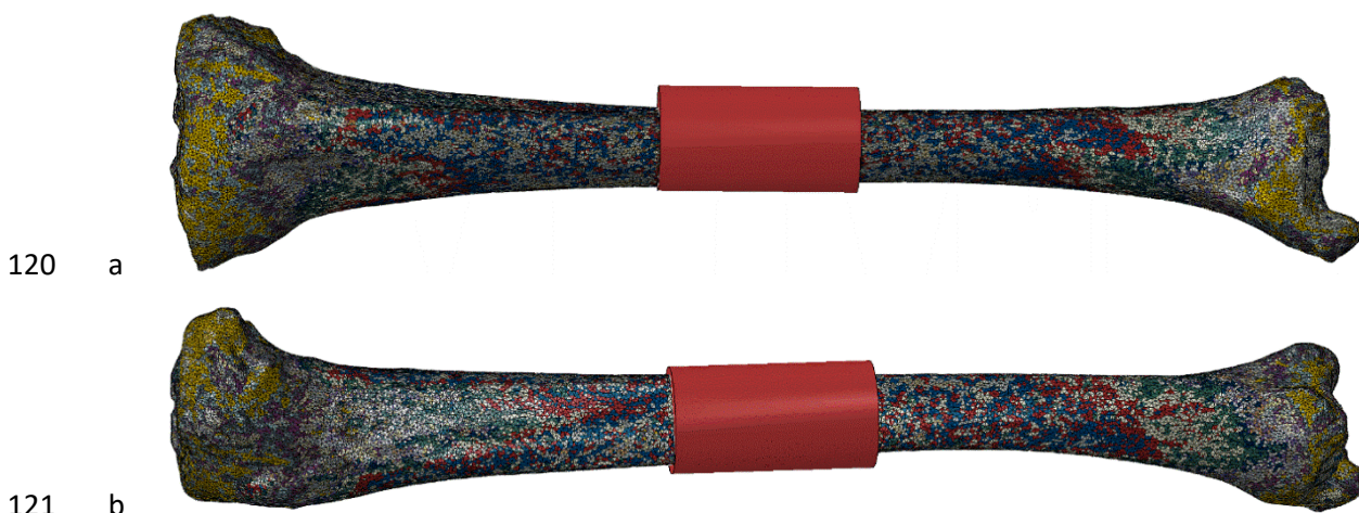
122 Figure 1: Finite element model of the tibia with a biomaterial colored in red implanted in a large 123 diaphyseal lesion. Views of the model in the front (a) and the sagittal (b) plane.
