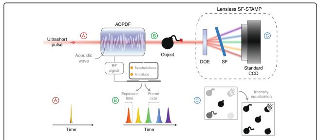
**Fig. 1 Principle of operation.** The acousto-optics programmable dispersive filter (AOPDF) tailors the pulse shape in both the spectral and temporal domains via its interaction with an electrically driven acoustic wave, then enabling the full and independent control over the exposure time and frame rate in the subsequent SF-STAMP detection scheme, comprising a diffractive optical element (DOE), a tilted spectral filter (SF) and a standard camera.
