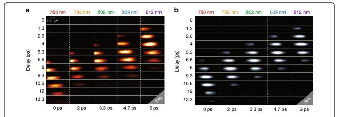
Fig. 4 Imaging of an optical Kerr gate (OKG) in the picosecond regime. a Vertically stacked images of the transmitted pulses while varying the optical delay. The opening and closing of the OKG are fully acquired for a delay of 6.6 ps. b Numerical simulation (see "Methods") of the OKG imaging process.
