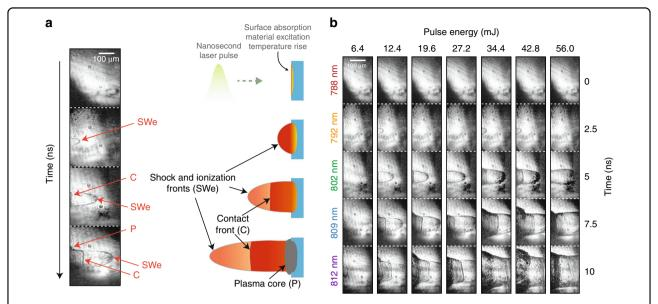
**Fig. 5 Capture of laser-induced ablation dynamics in the nanosecond regime. a** Birth and evolution of laser-induced gas dynamics captured using our system and illustration of the physical phenomena involved. The shock and ionization front (external shock wave, SWe), as well as the contact front evolution, are clearly observed. **b** Monitoring of gas dynamics during laser ablation on glass while varying the pump pulse energy.
